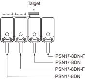
When installing several proximity sensor closely, it may cause malfunction due to mutual interference. Therefore, please use differential frequency for the application %Differential frequency type is only for 17 square.
