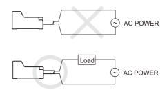
When using DC 2-wire and AC 2-wire type, a load must be connected before applying power; otherwise, components can be damaged.
